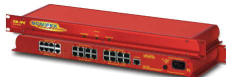
RB-IPE IP Extender for GPIO & Analogue Control Signals.
