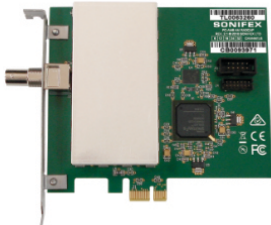
PC-AM 6-32 AM Stations Radcap PCIe Card.
