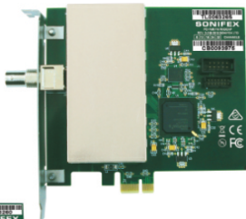
PC-AM 6-32 AM Stations Radcap PCIe Card.
